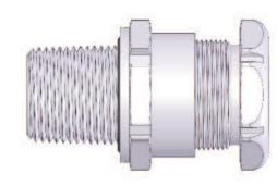
2. Slacken the seal nut (5) to relax the seal. Try to pass the cable through the connector. If this is possible, move to stage 3.
