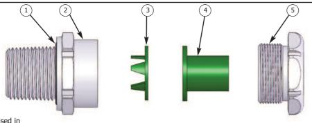
Note\*: The Seal and Nut inserts are only used in connector sizes 40 (1-1/4") and below to give two cable size ranges.
